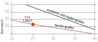
PREN = % Cr + 3.3% Mo + 16% N for austenitic steel. PREN = % Cr + 3.3 % Mo for ferritic steel.
