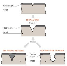
This dissolution gives rise to metal ions and electrons and thus the passage of current (of dissolution) which gives rise to an electrical potential difference between the anodic zone (pitting) and the cathodic zone (the rest of the metal).
