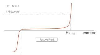
The pitting potential corresponds to the potential necessary to initiate stable pits.
