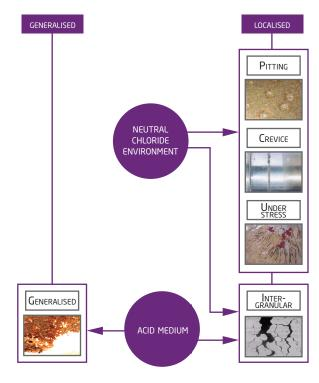
Generalised corrosion is noticed when stainless steel is in contact with an acid medium and localised corrosion is seen in the majority of cases when stainless steel is placed in a neutral chloride environment
