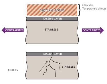
The metallurgical structure of stainless steels influences their behaviour in this type of configuration.
