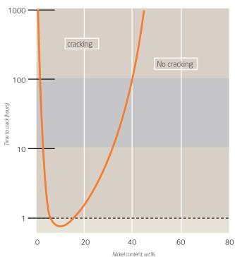
Effect of nickel content on the resistance to stress corrosion of
