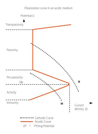
In a low oxidising medium, the cathodic curve (M) cuts the anodic curve below the pitting potential: metal remains intact.
