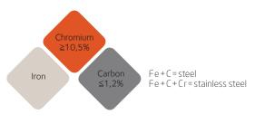
Indeed, on contact with oxygen, a chromium oxide layer is formed on the surface of the material. This passive layer protects it and has the particular ability to self repair.
