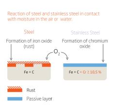
However if this protective layer is damaged, the start of corrosion can appear
