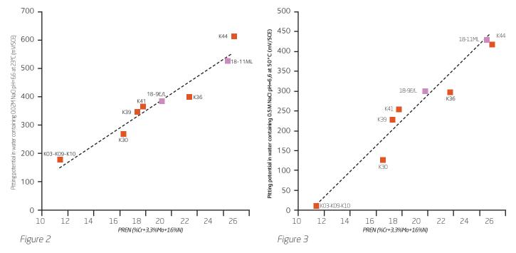
In order to map the duplex range, tests in the most severe medium, 0.5M NaCl (17.75g/I Cl<sup>-</sup>) at 50°C, were carried out. The results obtained are shown below.
