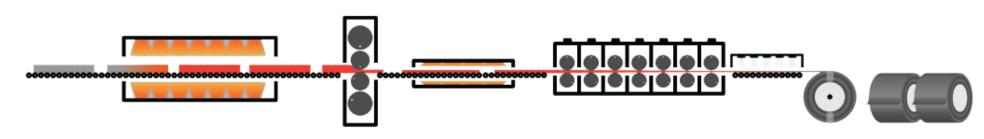
This process takes place at **Aperam Châtelet** and initially involves slab reheating in a furnace at an average temperature of 1250 ° C.
