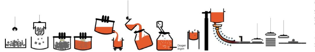
The raw material - recycled stainless steel and ferro-alloys - is transformed into molten metal in an electric arc furnace with a melting capacity up to 160 tonnes.
